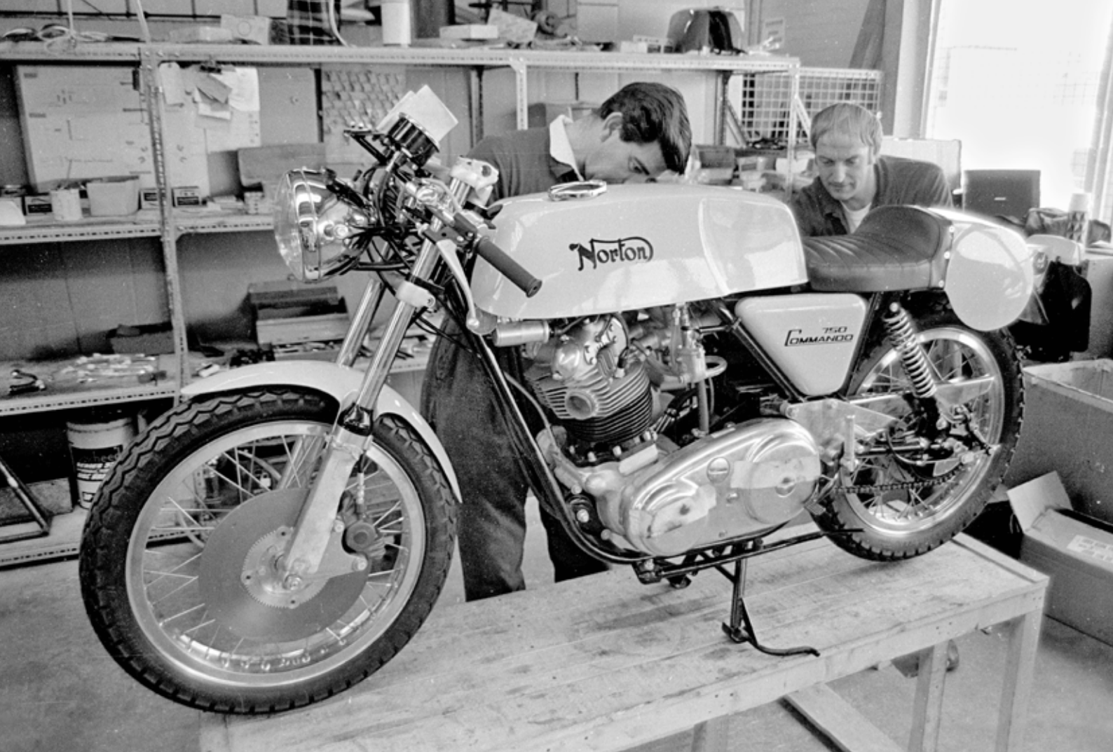
Norton workers build a Commando production racer. This particular machine must be a special order, because at the time the production racer had been discontinued. It is probably being assembled with leftover parts. It all looks to be in order, except the sidestand and bracket which would make the tug-in exhaust headers of the production racer impossible to fit. Production racers weren't delivered with sidestands. Also none had the notorious '72 crankcases.
